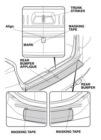
6. Remove the backing shown. Using the applicator with the soft sleeve, apply pressure to smooth out the top surface the rear bumper applique. If you see any air bubbles, gently peel up that section and work out the air bubbles.
