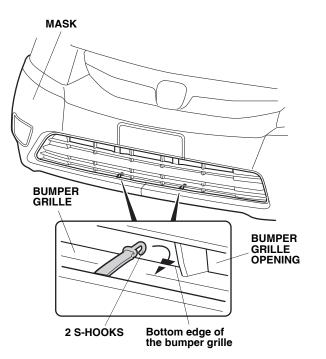
Route the elastic cord through the ten loops on the bottom of the mask. Attach one S-hook to the bottom edge of the bumper on one side. Stretch out the cord after routing it through each
