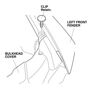
3. Install one new clip with a snap-screw into the hole where you removed the clip, and tighten the snap-screw.
