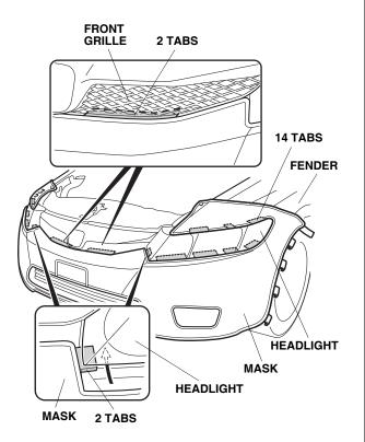
9. Pull the mask back toward the wheelwell, smooth out any wrinkles, and attach the four plastic hooks to the fenderwell, then bend the metal tab around the fenderwell. Repeat on the other side.
