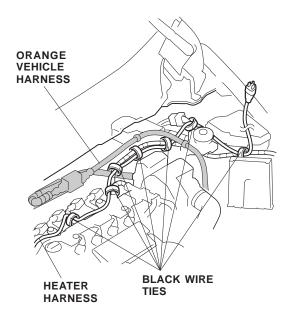
14. Continue routing the heater harness down below the fan shroud.
