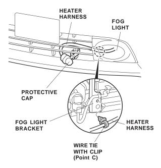
18. Attach the protective cap to the grille, and plug the heater harness connector into the protective cap.
