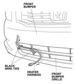
22. Attach the protective cap to the front bumper grille, and plug the connector of the heater harness into the protective cap. Go to step 25.
