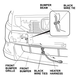
24. Attach the protective cap to the front bumper grille, and plug the connector of the heater harness into the protective cap.
