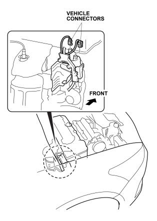
10. Release the vehicle harness holder from the vehicle bracket (two hooks).
