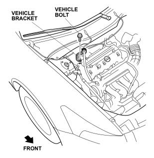
7. Disconnect the vehicle connector from the ABS or VSA Modulator, and release the harness clip from the vehicle bracket.
