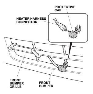
23. Route the heater harness inside the bumper, and secure it with the three black wire ties.
