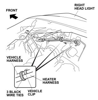
20. Route the heater harness as shown, and secure the wire tie with clip (points G) to the vehicle frame.
