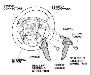
Reinstall the two self-tapping screws to the steering wheel.
