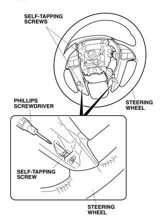
Remove the self-tapping screw that fastens the left steering wheel trim and the right steering wheel trim from the steering wheel, and unplug the switch connectors.
