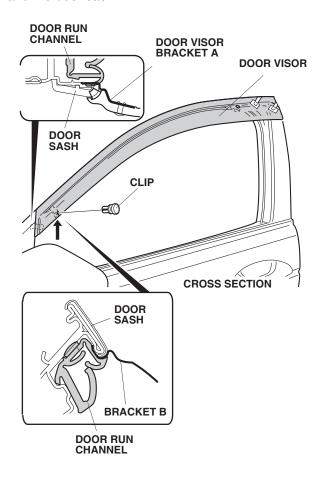
8. Adjust the position of bracket C to install the door visor, then install the clip. Push up on bracket C so the door run channel fit tightly to the bracket. There should be no clearance between the bracket and the door sash.
