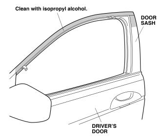
6. Position the door visor on the door sash.
