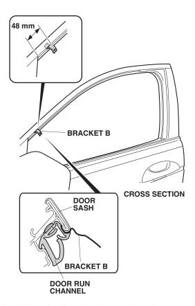
Install bracket B to the door sash at the measurement shown. Verify the shape at the identification mark stamped on the bracket. Be sure the door run channel is installed properly before installing the bracket.  Install bracket C on the door sash at the measurement shown. Verify the shape and the identification mark stamped on the bracket. Be sure the door run channel is installed properly before installing the bracket.
