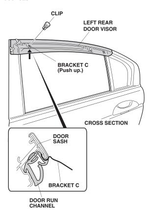
18. Measure the distance between the edge of the door visor and the outside edge of the door sash as shown.
