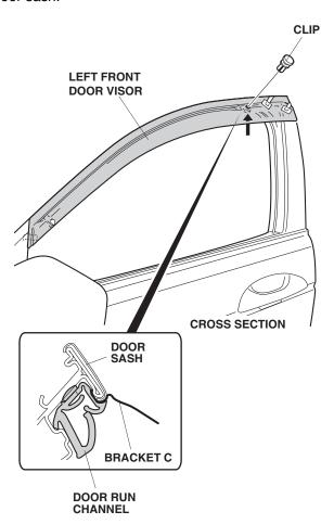
9. Measure the distance between the edge of the door visor and the outside edge of the door sash as shown.
