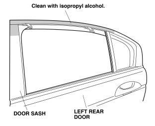
15. Position the door visor on the door sash.
