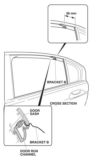
11. Install bracket B to the door sash at the measurement shown. Verify the shape and the identification mark stamped on the bracket. Be sure the door run channel is installed properly before installing the bracket. 12. Install the bracket C to the door sash at the measurement shown. Verify the shape and the identification mark stamped on the bracket. Be sure the door run channel is installed properly before installing the bracket.
