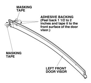
5. Using isopropyl alcohol on a shop towel, clean the door sash where the left front door visor will attach.
