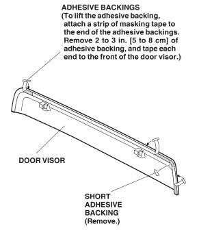
Push the two door visor brackets onto the door sash.
