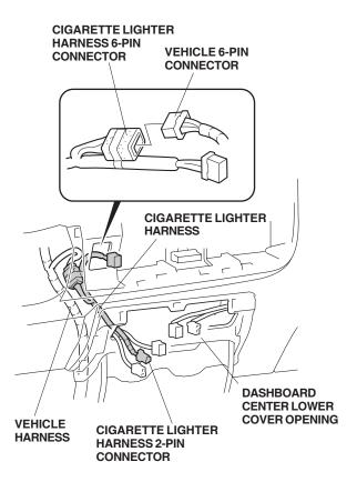
12. Connect the vehicle 2-pin connector and cigarette lighter harness 2-pin connector into the socket of the cigarette lighter. Reinstall the dashboard center lower cover.
