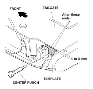
10. Using the felt-tip pen and the center punch, mark the right side of the tailgate at the center of the triangle area.
