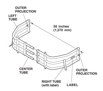
4. Adjust the tubes so that the distance between the outer projections on the ends of the right and left tubes are 50 inches (1,270 mm).
