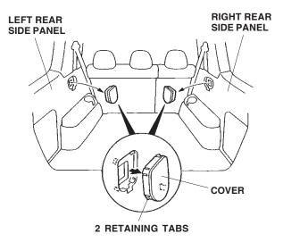
Install the cargo cover into the recess in the left rear side panel in the direction shown, then compress the cargo cover, and install it in the right rear side panel.
