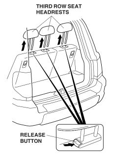
Store the headrests in the storage compartment under the cargo floor. Insert the posts of the headrests into the holes in the front of the storage compartment.
