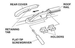
2. Insert two holders in the groove of the roof rail.
