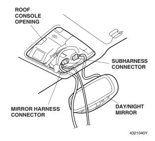
23. Attach the mirror harness connector to the vehicle panel with one EPT sealer as far forward as possible.
