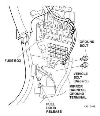
33. Secure the mirror harness to the vehicle harness using two wire ties.
