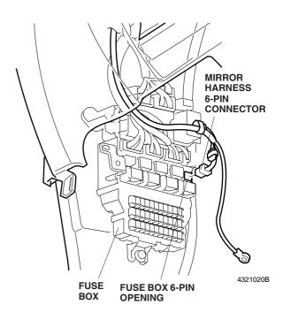
NOTE: If another accessory is already plugged into the 6-pin connector, remove the dummy connector from the 6-pin connector taped to the day/night harness. Plug the 6-pin connector from the other accessory harness into the 6-pin connector from the day/night harness you just unplugged, and plug the day/night harness into the fuse box.
