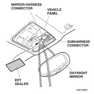
24. Route the terminal from the mirror harness under the headliner toward the right side of the vehicle.
