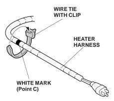
Plug the connector of the heater harness into the engine block heater, and route the heater harness over the engine. Secure the heater harness to the vehicle harness with one white wire tie in the area shown.
