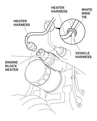
Route the heater harness alongside the vehicle harness, and secure the heater harness to the sensor connector and the vehicle harness with two white wire ties in the areas shown.
