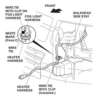
17. Secure the heater harness to the hole in the front side frame with the black wire tie.
