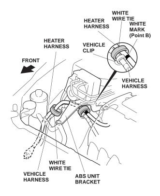
11. Route the heater harness to the back of the right headlight along the vehicle harness, then secure the harness with one black wire tie in the area shown.
