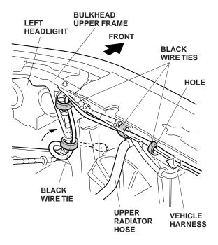
15. Secure the heater harness to the vehicle harness with three black wire ties. At the upper radiator hose area, secure the heater harness next to the existing vehicle wire tie.
