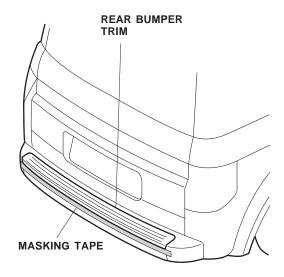
Using isopropyl alcohol on a shop towel, clean the rear bumper where the trim will attach.
