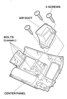
10. Loosen the four bolts on the right and left audio brackets.
