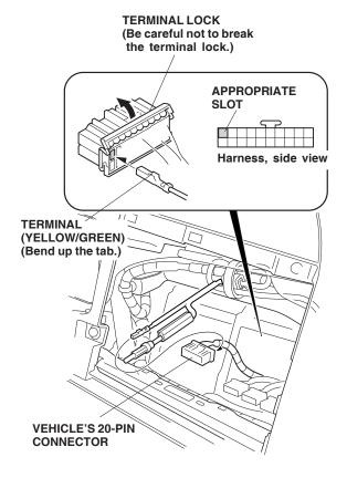
15. Carefully push the wire terminal (yellow/green) of the antenna subharness into the appropriate slot of the vehicle 20-pin connector. Reattach the terminal lock.
