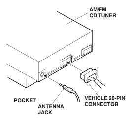
21. Connect the vehicle connectors to the center panel, and reinstall the center panel.
