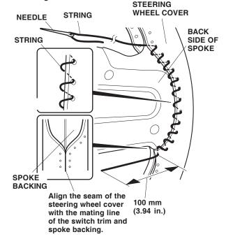
8. After lacing the string through the holes in the steering wheel cover at the back side of the spoke, pull the string tight so the cover wrinkles slightly at the edge. Best fitment results are obtained by lacing up the steering wheel cover tightly.
