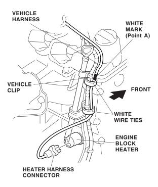
12. Secure the heater harness to the vehicle harness using two white wire ties. Attach one wire tie at the white mark (point A) made in step 8.
