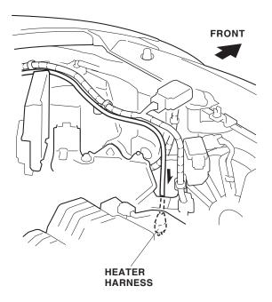
15. Secure the wire tie with clip that you installed on the heater harness at point B to the vehicle frame. Route the heater harness to the front bumper opening.
