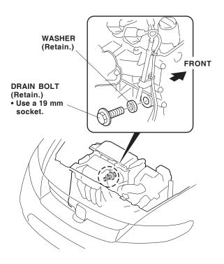
Install the new aluminum washer and the engine block heater into the bolt hole using a 24 mm socket and a torque wrench. Torque the engine block heater to 60 N·m (6 kg.m, 44 lb-ft).
