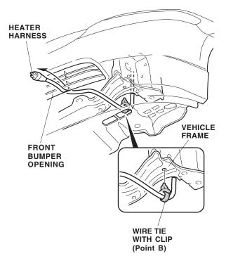
16. Secure the heater harness to the vehicle harness using three black wire ties.
