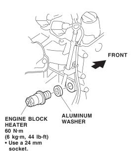
11. Route the heater harness down to the engine block heater, and plug the heater harness connector to the engine block heater.
