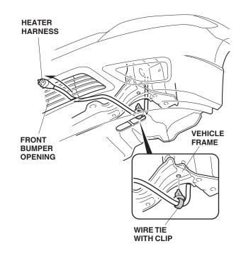
21. Secure the heater harness to the vehicle harness using five black wire ties.
