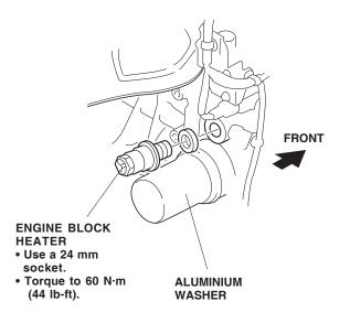
15. Route the heater harness down to the engine block heater. Connect the heater harness connector to the engine block heater.
