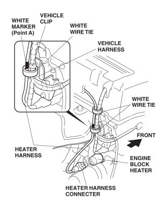
16. Secure the heater harness to the vehicle harness with one white wire tie at the marked point A. Then secure the heater harness to the vehicle harness, using another white wire tie above the point marked A. 17. Secure the heater harness to the vehicle harness with one black wire tie at the marked point B.
