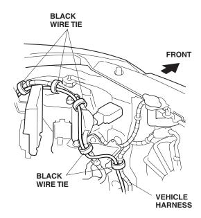
22. Route the heater harness on the inside of the bumper opening and secure it to the grille with two black wire ties.
