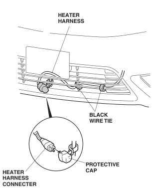
23. Attach the protective cap to the grille, and plug the heater harness connector into the protective cap.
