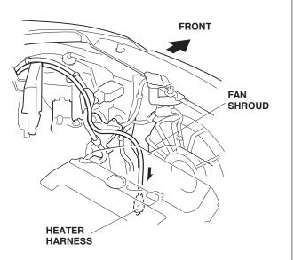
20. Secure the wire tie with clip (installed on the heater harness in step 10) to the vehicle frame, and route the heater harness to the front bumper opening.
