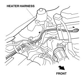
19. Route the heater harness through the engine compartment as shown.
