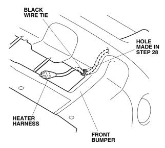
31. Install the protective cap on the heater harness connector.
