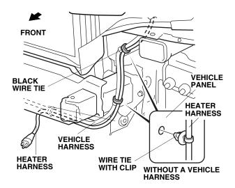
23. If the vehicle is not equipped with a vehicle harness, secure the heater harness to the vehicle panel using two wire ties with clip as shown.
