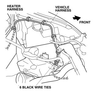
25. Secure the heater harness to the vehicle harness using one white wire tie and five black wire ties in the areas shown.
