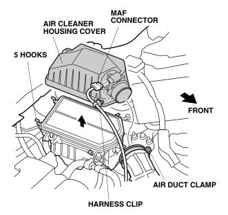
10. Remove the air cleaner housing (two bolts and one pin).
