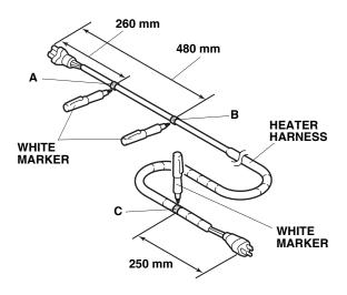
15. Plug the heater harness into the engine block heater.
