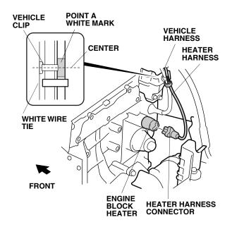
16. Using one white wire tie, secure the heater harness to the vehicle harness at the point A mark on the harness.
