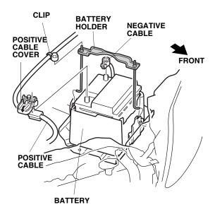
8. Remove the battery cover, battery, and battery tray.
