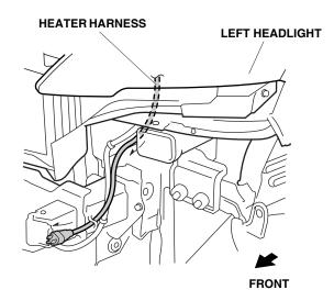
21. Continue routing the engine block harness under the bumper beam. Using one black wire tie, secure the heater harness to the vehicle harness at the point C mark on the harness.
