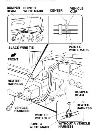
22. Secure the heater harness to the vehicle harness using two black wire ties as shown.
