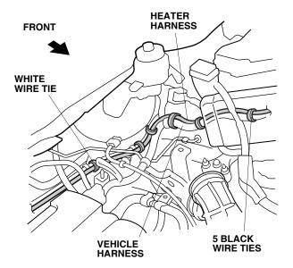
26. Secure the heater harness to the vehicle harness using two white wire ties in the areas shown.
