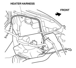
20. Route the heater harness through the front bulkhead as shown.
