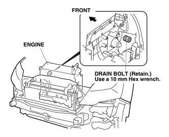
13. Install the new aluminum washer and the engine block heater into the bolt hole using a 24 mm socket and a torque wrench. Torque the engine block heater to 60 N·m (44 lb-ft).
