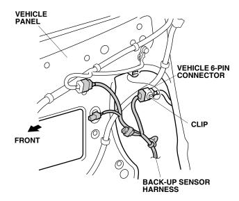
Secure the other 6-pin connector to the vehicle harness with one wire tie.
