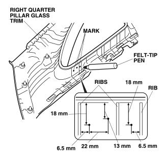
29. While wearing eye protection, drill a 4 mm hole at the two marked points, and remove any burrs.
