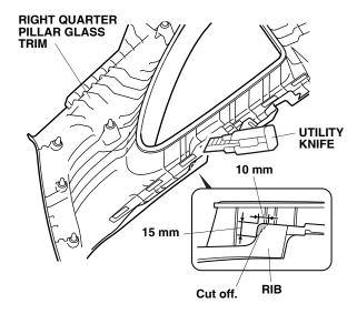
28. Using a ruler and a felt-tip pen, measure and mark the right quarter pillar glass trim in the area shown.
