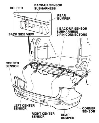
50. Attach the holder of the back-up sensor subharness to the rear bumper as shown.
