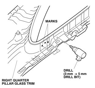
30. While wearing eye protection, drill a 3 mm bit, drill a hole at the marked point, then finish with a 16 mm hole saw. Remove any burrs.
