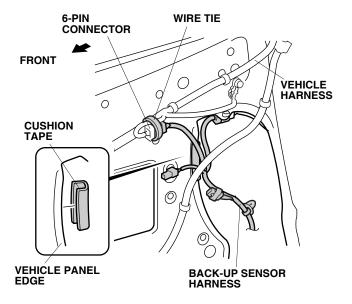
21. Using isopropyl alcohol on a shop towel, thoroughly clean the area where the cushion tape will attach. Attach the cushion tape to the edge of the vehicle panel at the location shown. 22. Slide the control unit bracket onto the control unit. Make sure that the three switches are in the down position.
