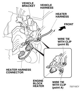
14. Route the heater harness as shown, and secure the wire tie with clip (point C) to the vehicle frame.
