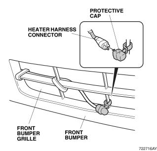
23. Route the heater harness inside the bumper, and secure it with the three black wire ties.
