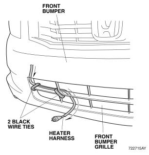
22. Attach the protective cap to the front bumper grille, and plug the connector of the heater harness into the protective cap. Go to step 25.
