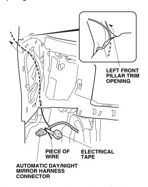
24. Remove the electrical tape and wire from the automatic day/night mirror harness.
