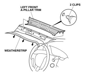
Remove and discard the clip from the left front A-pillar trim, and install a new clip (supplied) to the trim.
