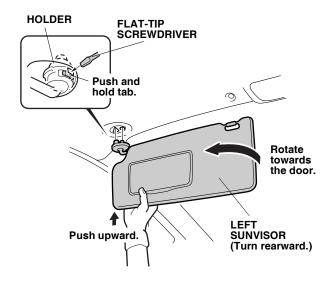
While holding the retaining tab, push up on the left sunvisor and rotate towards the door to remove the sunvisor. Disconnect the vanity mirror light connector.
