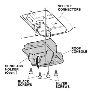
6. Turn the sunvisor holder 45°, and remove the two sunvisor holders.
