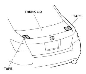
7. Close the trunk lid. Align the template with the edge of the trunk lid on the left side. Using a felt-tip pen, mark the trunk lid as shown on the template. Remove the template.
