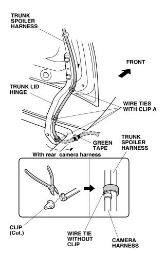
29. Route the trunk spoiler harness, and secure it to the vehicle panel holes with two wire ties with clip.
