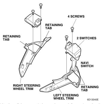
13. Install the two switches to the new left steering wheel trim and new right steering wheel trim with the four screws (reuse). Make sure the retaining tabs are engaged. Go to step 16.
