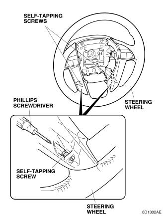
Remove the self-tapping screw that fastens the left steering wheel trim and the right steering wheel trim from the steering wheel, and unplug the switch connectors.
