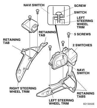
15. Install the two switches and NAVI switch to the new left steering wheel trim and new right steering wheel trim with the five screws (reuse). Make sure the retaining tabs are engaged.
