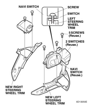
Connect each switch connector and install each new steering wheel trim to the steering wheel with the two screws you removed.
