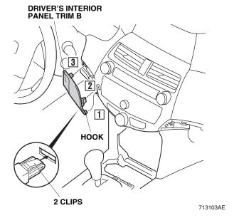
6. Install passenger's interior panel trim (eight clips and one hook). Install in the order shown. 1→2→3
