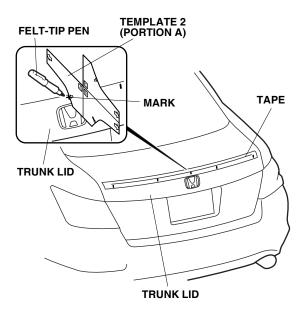
5. Position template 2 (portion B) on the inboard marks. Using a felt-tip pen, mark the tape at the notches shown.
