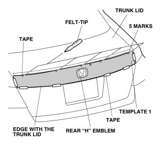
4. Position template 2 (portion A) on the trunk lid at the center mark. Using a felt-tip pen, mark the tape at the notch shown.
