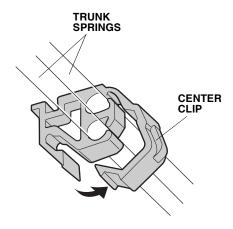
15. With an assistant holding the trunk lid open, remove the right trunk spring from the trunk hinge arms using the trunk spring tool. Wear gloves to protect your hands, and pull the trunk spring tool slowly and carefully towards you. Do not remove the left trunk spring.
