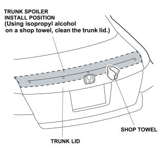
Insert stud bolts from the trunk spoiler into the 8 mm holes in the trunk lid. Install the five washer nuts to the stud bolts, but do not tighten the five washer nuts yet.
