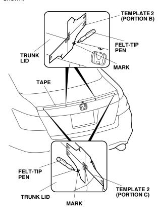
6. Position template 2 (portion C) on the outboard marks. Using a felt-tip pen, mark the tape at the notches shown.
