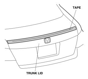
3. Close the trunk lid. Align template 1 with the rear "H" emblem and edge with the trunk lid. Tape template 1 to the trunk lid. Using a felt-tip pen, mark the trunk lid as shown on the template. Remove the template.
