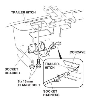
27. Remove the dummy connector from the vehicle 10-pin connector, and plug the socket 10-pin connector into the vehicle 10-pin connector.
