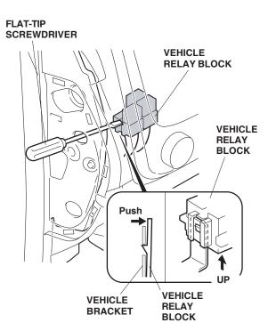
14. Install a relay into the vehicle relay block, and reinstall the vehicle relay block.
