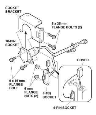
25. Remove the cover from the 4-pin socket, and install the 4-pin socket to the socket bracket with two 6 x 35 mm flange bolts and two 6 mm flange nuts. Reattach the cover.
