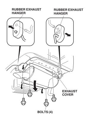
19. Remove the four bolts, and slide the exhaust cover around the muffler to allow access to the trailer hitch mounting holes.
