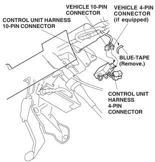
10. Plug the vehicle 10-pin and 4-pin connectors (if equipped) into the control unit harness 10-pin and 4-pin connectors.
