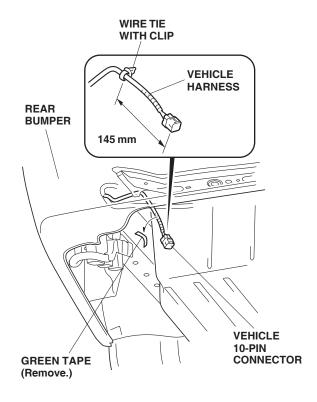
16. Measure from the end of the harness, and attach one wire tie with clip to the vehicle harness as shown.
