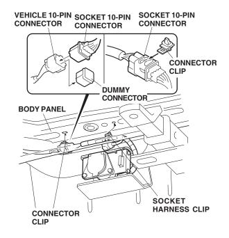
28. Install the connector clip into the vehicle 10-pin connector, and push the connector clip and socket harness clip into the holes in the body panel.
