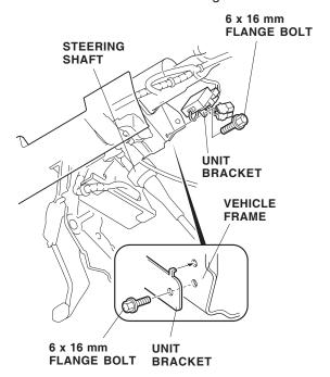
12. Install the relay block on the control unit harness to the unit bracket.
