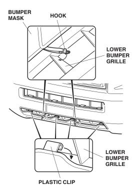
16. Attach the six hooks to the bottom inside edge of the front bumper.
