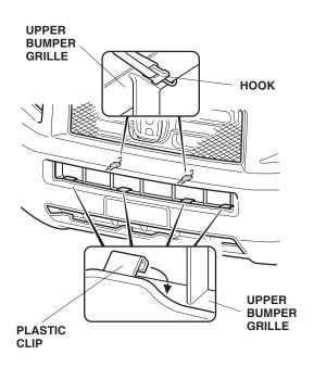
15. Attach the four plastic clips and the two hooks to the lower bumper grille.
