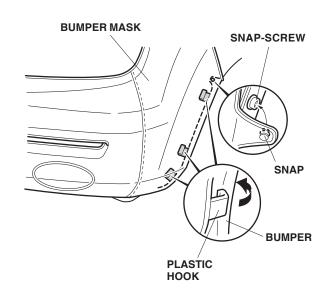
13. On both sides of the vehicle, attach the three plastic hooks to the fenderwell.
