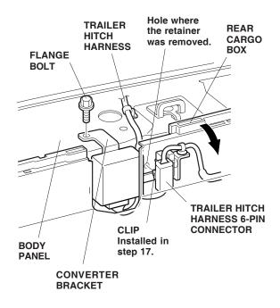
24. Align the hole in the converter bracket with the hole in the body panel and install the flange bolt.
