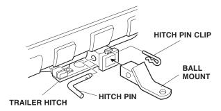
39. Slide the hitch pin through the trailer hitch and ball mount, then install the hitch pin clip in the hole in the end of the hitch pin.
