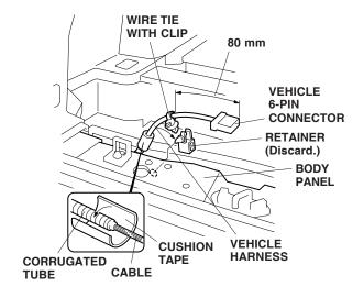
9. Attach one wire tie with clip to the vehicle harness in the area shown. Wrap one cushion tape around the joint section between the corrugated tube of the vehicle harness and cable.
