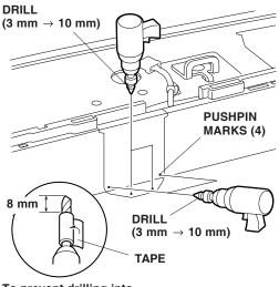
To prevent drilling into the frame, apply tape to the end of the drill bit
