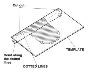
11. On the driver's side of the vehicle near the vehicle harness, tape the template inside the rear cargo box in the area shown.
