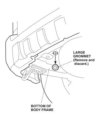
6. Inside the vehicle, locate the grommet on the body panel. Remove and discard the grommet from the body panel.
