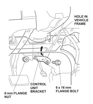
17. Install the control unit to the control unit bracket.
