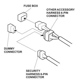
Secure the security harness to the vehicle harness with one wire tie.
