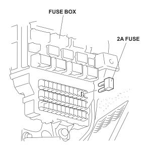
27. Attach the 2A fuse label to the No. 33 slot on the fuse box cover.
