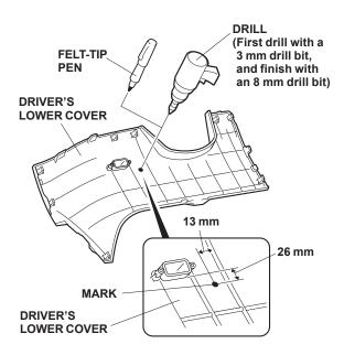
20. While wearing eye protection, drill an 8 mm hole through the marked location. First drill with a 3 mm drill bit, then finish with an 8 mm drill bit. Remove any burrs. 21. Route the microphone cable through the hole in the driver's lower cover, and seat the microphone flush in the cover.
