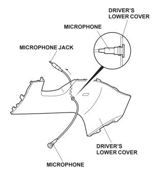
22. Attach a wire tie clip the microphone cable at the indicated position.
