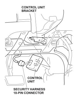
Plug the security harness 18-pin connector into the control unit.
