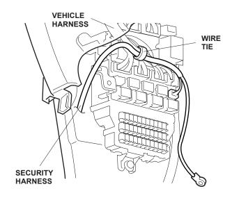
11. Route the ground terminal from the security harness down below the fuse box.
