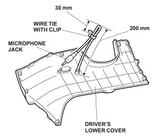
23. While holding the driver's lower cover near the dashboard, attach the wire tie with clip into the vehicle bracket.
