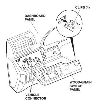
9. Remove the passenger's console panel (six clips), and install the wood-grain console panel.
