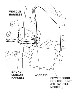
31. Plug the backup sensor harness 5-pin connector into the buzzer unit. Attach the backup sensor harness to the vehicle panel using two wire ties with clips.
