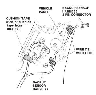
Using the remaining half of the cushion tape, secure the backup sensor harness to the vehicle's panel. 34. Using isopropyl alcohol, clean the areas where the cable clips will attach. On the outside of the vehicle, route the backup sensor harness across the back of the vehicle. Secure the backup sensor harness to the vehicle panel and to the bumper beam with two cable clips and two small wire ties.
