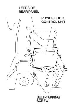
14. At the left rear panel area, enlarge the panel hole to 8 mm. While wearing eye protection, drill the body panel using an 8 mm drill bit and a drill stop.
