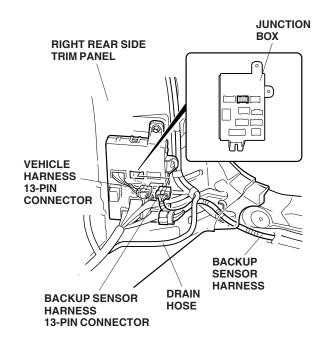
23. Route the backup sensor harness under the drain hose, and secure the backup sensor harness to the vehicle harness with two wire ties.
