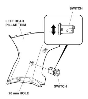
41. Plug the backup sensor harness 3-pin connector into the switch, and reinstall the left rear pillar trim.
