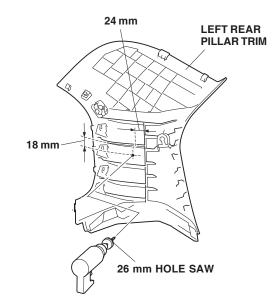
40. Install the switch into the hole in the left rear pillar trim in the direction shown.
