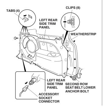
12. Remove the left rear pillar trim (one cover, one bolt, one clip, two tabs).
