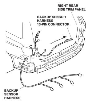
21. Pull the weatherstrip away from the right rear side trim panel. Remove the one anchor screw, and gently pull out on the trim panel to release the two clips.
