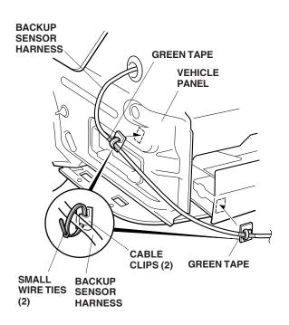
35. Using scissors, cut two EPT sealers in half. Attach one cut EPT sealer piece at each green tape location on the backup sensor harness.
