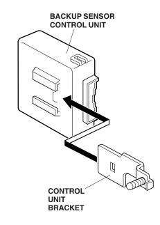
29. Plug the backup sensor harness 10-pin connector into the control unit. Attach the control unit to the inside of the left rear vehicle panel using one 6 mm flange nut.
