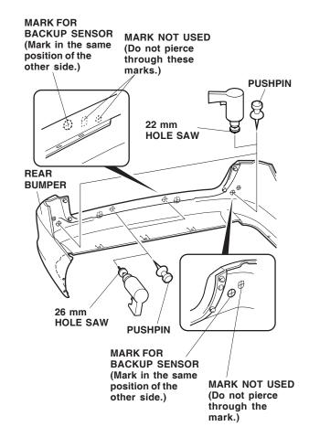
43. While wearing eye protection, drill a 22 mm hole through the outboard marks, and drill a 26 mm hole through the two inboard marks. Remove any burrs.
