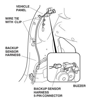
32. Install the two wire ties with clips to the vehicle panel.
