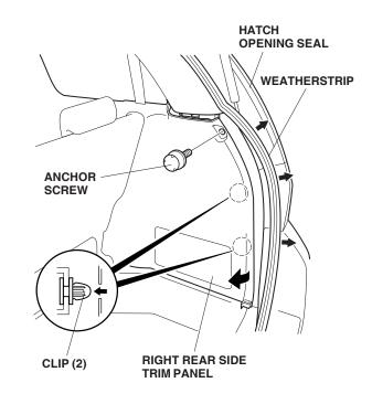
22. Behind the right rear side trim panel, disconnect the 13-pin connector from the junction box. Insert the 13-pin connector on the backup sensor harness into the junction box. Plug the vehicle harness 13-pin connector into the backup sensor harness.
