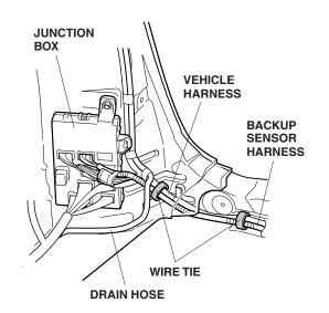
24. Secure the backup sensor harness to the vehicle harness with five wire ties.
