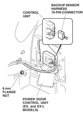
30. Secure the backup sensor harness to the vehicle harness using one wire tie.
