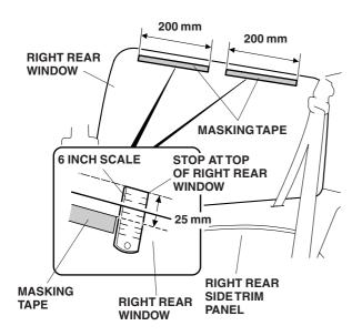
23. Pull up the rear sunshade until the cutouts in the sunshade reach the masking tape. Using a felt-tip pen, mark the top of the masking tape at each side of each cutout. Roll down the rear sunshade.
