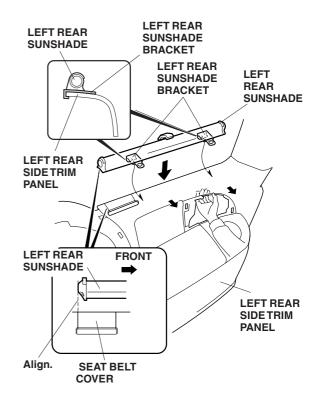
6. Using a felt-tip pen, mark the left rear side trim through the center of each bracket hole. Remove the rear sunshade.
