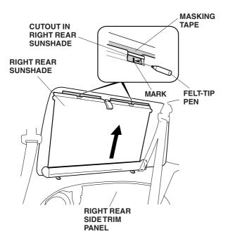
24. Using isopropyl alcohol on a shop towel, clean the right rear window above the marks you made on the masking tape.
