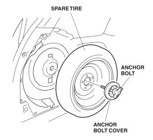
Pull away the weatherstrip from the left rear side trim panel. Remove the anchor bolt, disengage the three clips and the four retaining tabs, and pull out the rear portion of the left rear side trim panel.
