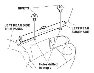
9. Secure the two brackets from the left rear sunshade to the left rear side trim panel with the two rivets. Reinstall the left rear side trim panel.
