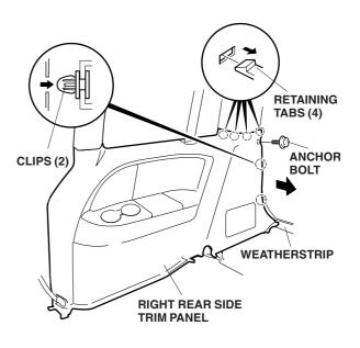
16. Remove the right rear speaker cover (two clips, and three retaining tabs).
