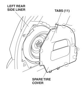
2. If equipped, remove the anchor bolt and the anchor bolt cover and take out the spare tire.
