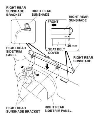
18. Using a felt-tip pen, mark the right rear side trim through the center of each bracket hole. Remove the rear sunshade.
