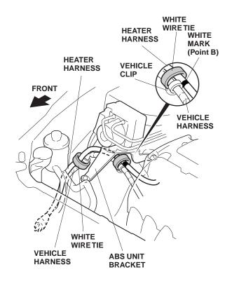
Route the heater harness to the back of the right headlight along the vehicle harness, then secure the harness with one black wire tie in the area shown.
