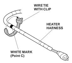
Plug the connector of the heater harness into the engine block heater, and route the heater harness over the engine. Secure the heater harness to the vehicle harness with one white wire tie in the area shown.
