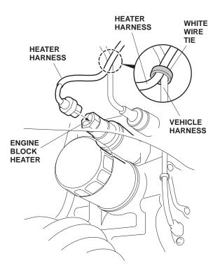
Route the heater harness alongside the vehicle harness, and secure the heater harness to the sensor connector and the vehicle harness with two white wire ties in the areas shown.
