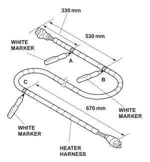
7. **Without the Fog Lights**: Install one wire tie with clip on the heater harness in the area shown.
