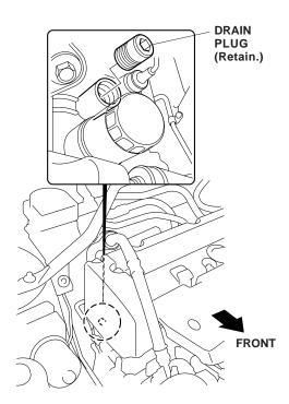
5. Install the engine block heater with the aluminum washer into the bolt hole using a 24 mm socket and a torque wrench. Torque the engine block heater to 60 N·m (44 lb-ft).
