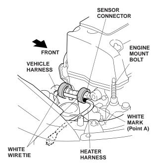
10. Continue routing the heater harness under the ABS unit bracket along the vehicle harness, and secure the heater harness to the vehicle harness with two white wire ties in the areas shown.
