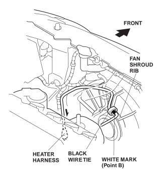
Secure the wire tie with clip, attached at point C, to the vehicle frame and route the heater harness to the front bumper opening.
