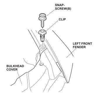
Repeat steps 2 and 3 to install a snap-screw(B) on the right side of the vehicle.
