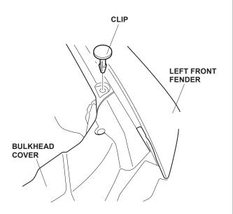
3. Install one new clip with a snap-screw(B) into the hole where you removed the clip, and tighten the snap-screw(B).
