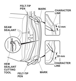
4. Position the hem sealant cutting tool against the door edge, and trim the seam sealant from mark to mark.
