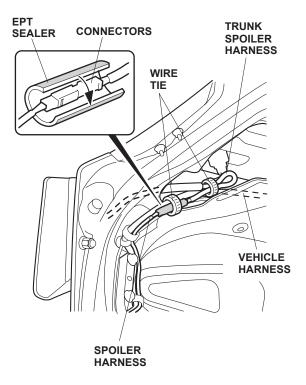
34. Make loops in the trunk spoiler harness, then secure the trunk spoiler harness and spoiler harness to the vehicle harness with the two wire ties as shown.
