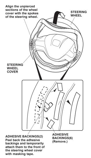
Turn over the steering wheel cover. Peel back the adhesive backings shown, and temporarily attach them to the front of the steering wheel cover with masking tape. Remove all the remaining adhesive backings from the steering wheel cover.
