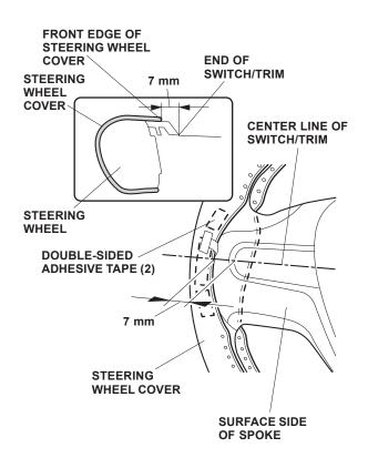
Align the rear edge of the steering wheel cover to the back of the steering wheel spoke as shown.
