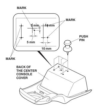
5. While wearing eye protection, drill four 5 mm holes and one 30 mm hole through the marks you just made.
