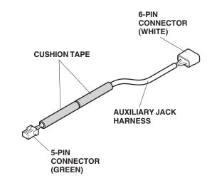
10. Locate the vehicle 6-pin connector blue taped to the vehicle connector. Remove the blue tape to free the connector. Plug the auxiliary jack harness 6-pin connector into the vehicle harness 6-pin connector.
