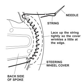
9. Tightly lace the string twice through the holes directly above the spoke as shown.
