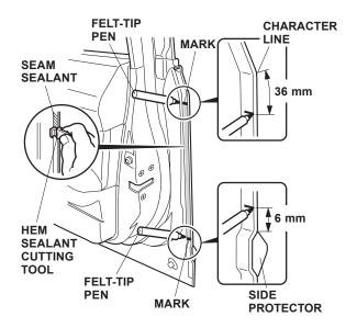
Position the hem sealant cutting tool against the door edge, and trim the seam sealant from mark to mark.
