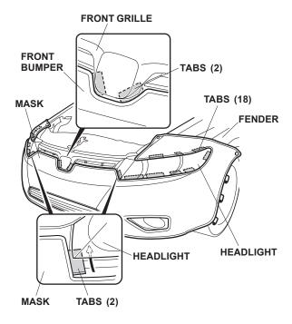
14. Pull the mask back toward the wheelwell, smooth out any wrinkles, and then snap the mask onto the snap-screw(A). Repeat on the other side.
