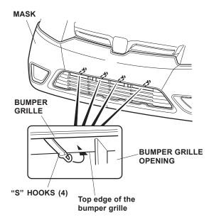
17. Attach the four plastic hooks to the bottom inside edge of the bumper grille opening.
