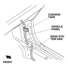
28. Secure the bass system harness to the vehicle harness using one wire tie.
