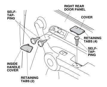
36. Remove the cover (four retaining tabs) and remove the self-tapping screw from the right rear door panel.
