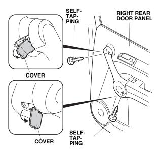
38. Pull the right rear door panel out toward you to release the seven clips, remove the inside handle from the door panel (three clips), disconnect the vehicle connector, and remove the right rear door panel.
