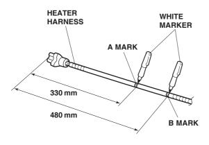
Plug the heater harness connector into the engine block heater, and secure the heater harness to the vehicle harness with one wire tie at the A mark.
