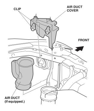
5. Remove the air duct (if equipped) by pulling it out toward you.
