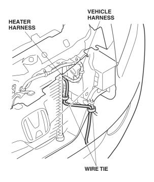
16. Fold the excess length of the heater harness, secure the heater harness to the vehicle harness with four wire ties.
