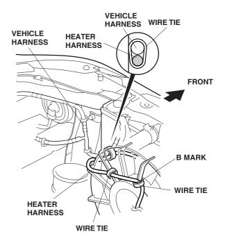
12. Secure the heater harness to the fan shroud and vehicle harness with two additional wire ties at the areas shown.
