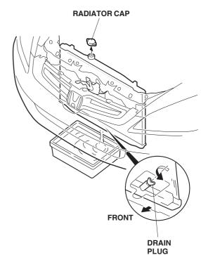
3. Remove the radiator cover (ten clips and four retaining tabs).
