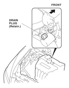
Install the engine block heater with the aluminum washer into the hole using a 24 mm socket.
