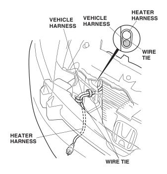
10. Secure the heater harness to the bumper grille with two wire ties.
