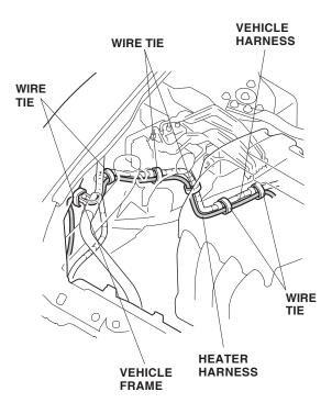
8. Continue routing the heater harness along the vehicle harness through the front bulkhead to the right side of the radiator. Secure the heater harness to the vehicle harness with two wire ties positioned on the inside of the front bulkhead.
