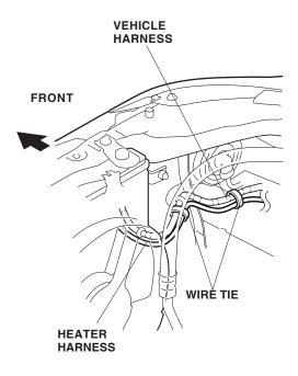
Secure the heater harness to the vehicle harness with two wire ties positioned on the outside of the front bulkhead.
