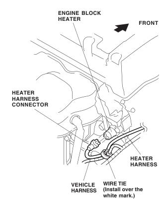
7. Route the heater harness alongside the vehicle harness, and secure the heater harness to the vehicle harness and frame with six wire ties.
