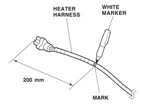
6. Plug the heater harness connector into the engine block heater. Route the heater harness along the vehicle harness, and secure it to the vehicle harness with one wire tie at the white mark.
