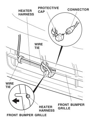
11. Attach the protective cap to the grille, and plug the connector of the heater harness into the protective cap.
