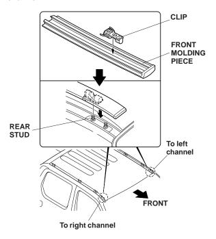
6. Reinstall all the molding you retained in step 4 in the roof channels.
