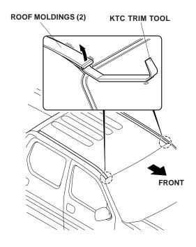
2. Slide up the end of the roof molding and remove the roof molding.
