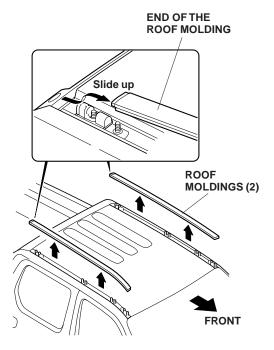
3. Remove the six clips from the roof channels.
