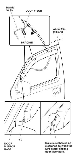
7. Check that the distance between the rear end of the door visor and front door is about 2 in. (50 mm).
