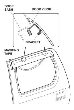
15. Align the front end of the door visor with the masking tape. While holding light pressure on the door visor, carefully remove the adhesive backing in the directions shown. Using the palm of your hand, hold the door visor firmly against the door for 30 seconds.
