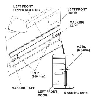
On the inside of the left front lower molding, attach
