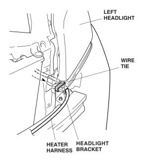
12. Route the heater harness along the front bumper beam and secure the heater harness to the bumper beam with seven wire ties.
