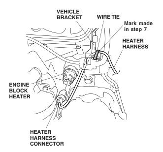
9. Route the heater harness along the fan shroud and secure the harness with three wire ties.
